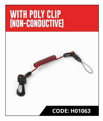
The Coil E-Tether With Poly Clip (Non-Conductive) is engineered to withstand harsh work environments and keep your small electronic devices secure at height. A heavy-duty nylon clip connects your phone, camera, radio or another electronic device to the tether anchor point, with a single-action poly clip swivel head that allows freedom of movement without tangles.
